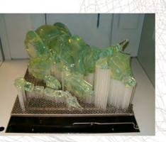
SLA is a fabrication process utilising a vat of liquid UV-curable photopolymer "resin" and a UV laser to build parts a layer at a time. On each layer, the laser beam traces a part cross-section pattern on the surface of the liquid resin. Exposure to the UV laser light solidifies the pattern traced on the resin and adheres it to the layer below.
